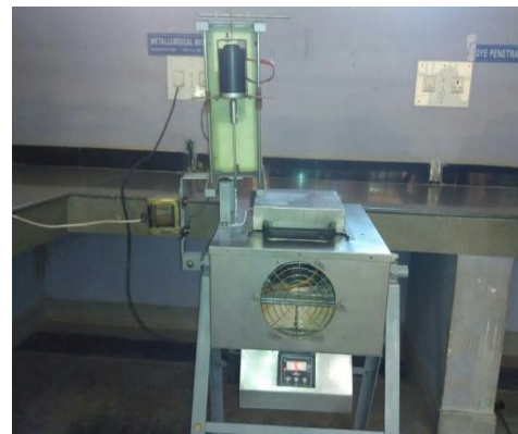
Figure 1. Stir casting setup.
