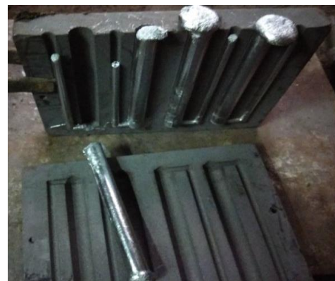
Figure 2. Al alloy composites in cast iron die.
